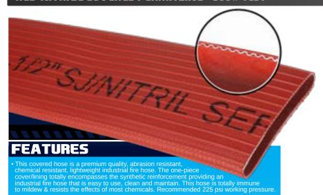
• Temp Range: -4° F to +174° F • Cover: Red, Nitrile Ш • Tube: EPDM • Reinforcement: White Polyester Jacke ASSEMBLIES p. 281
