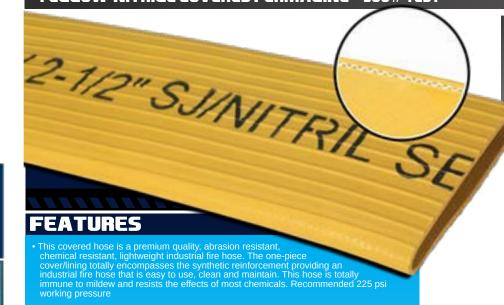
• Temp Range: -4° F to +174° F • Cover: Yellow, Nitrile П • Tube: EPDM • **Reinforcement:** White, Polyester Jacket ASSEMBLIES p. 281
