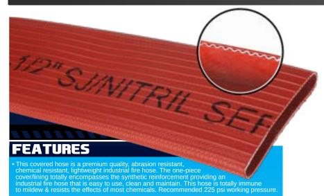
• Temp Range: -4° F to +174° F • Cover: Red, Nitrile Ш • Tube: EPDM • Reinforcement: White Polyester Jacke ASSEMBLIES p. 255
